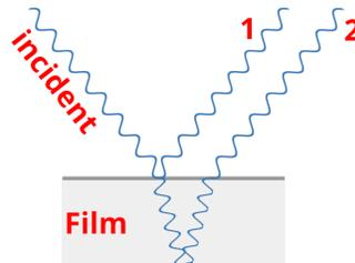
Under certain conditions, wave 1 and wave 2 will constructively interfere.
