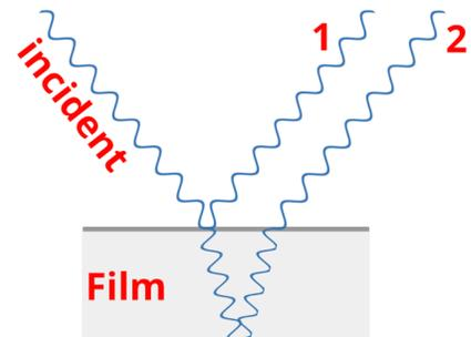
If Path Difference =  $1 \cdot \lambda$  or  $2 \cdot \lambda$  or  $3 \cdot \lambda$  or ... \*, then wave 1 will have its crests lines up with the crests of wave 2 (i.e., the two waves will be in phase).
