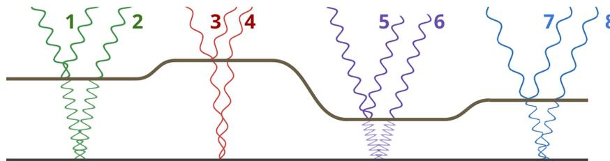
The thickness at different locations allows different wavelengths or colors to be intensified at those locations.
