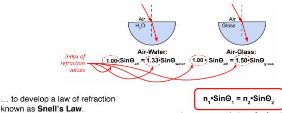
$n_1$  and  $n_2$  represent index of refraction values  $\Theta_1$  and  $\Theta_2$  are the angles of incidence and refraction
